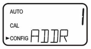
Select the operating mode either ASCII or RTU using the  $\uparrow$  or  $\checkmark$  buttons. Press the **MODE** key to complete the Modbus setup.
