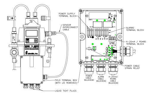
**Figure 1: Electrical Connections for the Instrument**
