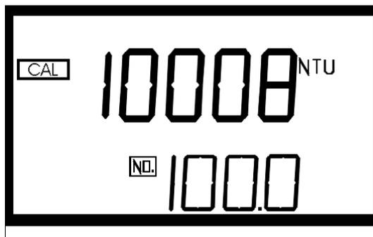
6. Insert the 100.0 NTU calibration standard into the sample well and calibrate as before. When the instrument has completed the calibration, the “Cal” and the “Store” blocks will quit flashing and the lower row of the display should now indicate that the 10.0 NTU standard is the next standard to be used for calibration.
