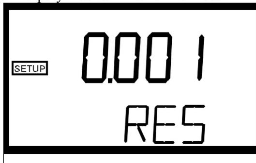
You have the ability to select the resolution shown on the display by pressing either the ▲ or ▼ keys to change the resolution to be used. When you have selected the desired resolution press the
