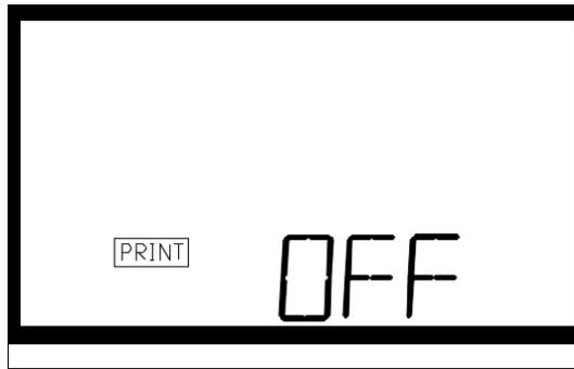
This feature allows you to select the function of the serial port on the instrument. There are two options to choose from: Off and Timed Output. Select the RS232 option by pressing either the ▲ or ▼ keys. When you have selected the proper function, press the
