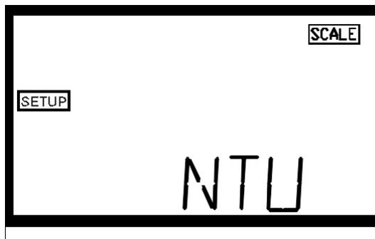
Press either the ▲ or ▼ keys to change the units that will be displayed during normal automatic measurement mode. When you have selected the desired units press the
