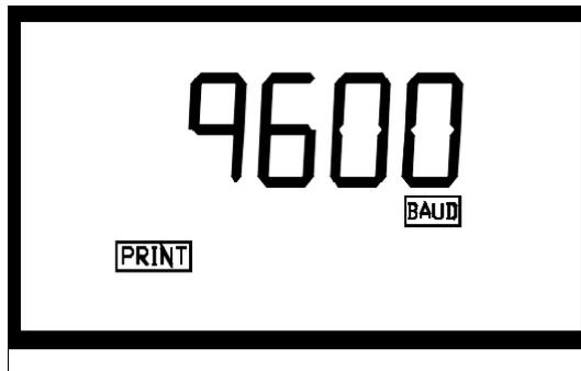
Select the desired baud rate (1200, 2400, 4800, or 9600) by pressing either the ▲ or ▼ keys to change the displayed baud rate. The other RS 232 parameters are fixed at 1 stop bit, 8 data bits and no parity. When you have selected the proper baud rate press the
