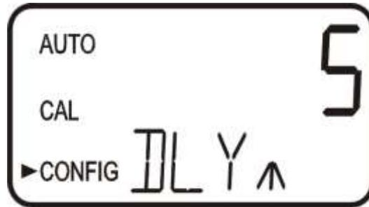
The current selected number of seconds will be shown. Select the desired number of seconds for the “delay on” time for this alarm using the  $\blacktriangle$  and  $\blacktriangledown$  buttons. Once the desired delay time has been set, press the  $\blacktriangleleft$  button to accept it.
