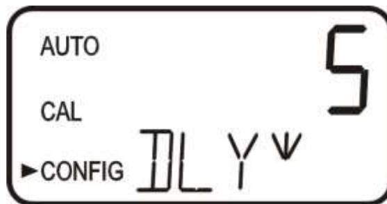
The current selected number of seconds will be shown. Select the desired delay off time for this alarm using the  $\blacktriangle$  and  $\blacktriangledown$  buttons. Once the desired delay time has been set, press the  $\blacktriangleleft$  button to accept it. After the settings for alarm 1 have been completed, prompts will allow for the set up of the information on alarm #2.
