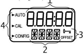
**Figure 1 – Display used in the instrument**. All items used on the display are shown in this figure
