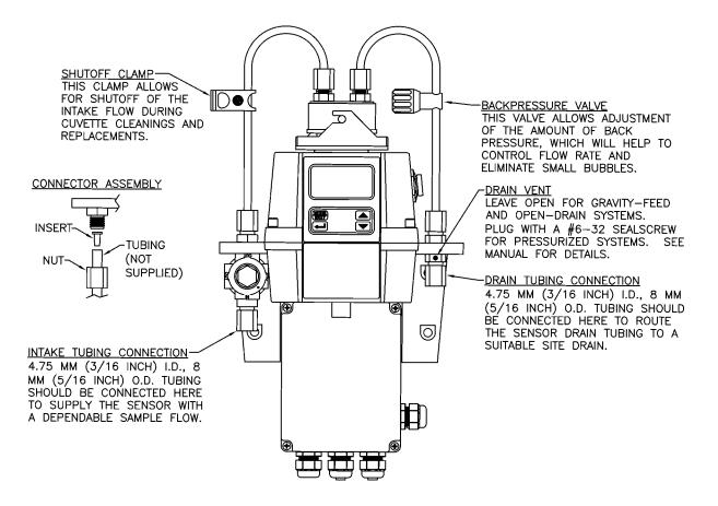
Figure 4: Recommended Plumbing for the Instrument
