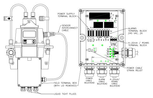
**Figure 5: Electrical Connections for the Instrument**
