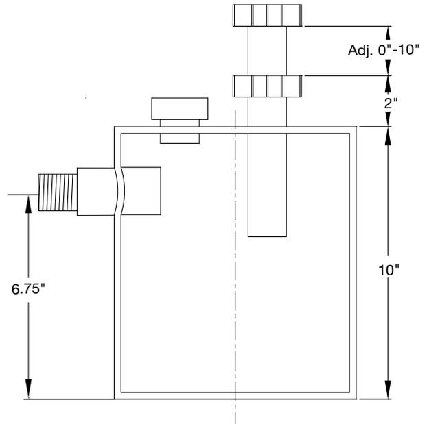
**Note:** Tanks are made to  $\pm 0.25$  in. tolerance.
