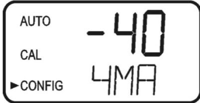
This setting will be slightly different on each instrument as each CLX-Ex2 will be factory set to 4.00mA. Press the ← button when adjustments are complete to save this setting and move on to the 20mA adjustment.
