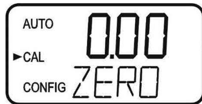
4. The screen will show the current reading on the CLX-Ex2. Since there is no chlorine, the only reading may be a slight offset due to the absorbance of the reagents. There should be no pink color developed.
