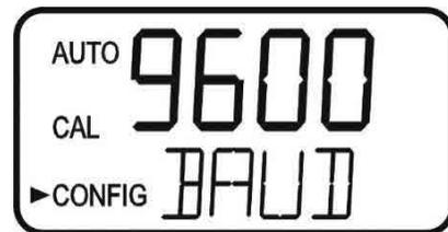
Select the correct baud rate (1200, 2400, 4800, 9600, or 19200) for operation of the I/O port by pressing the **▲** or **▼** buttons to change the displayed baud rate.
