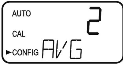
**Note:** This software filter is completely disabled when the averaging (AVG) is set to 1.
