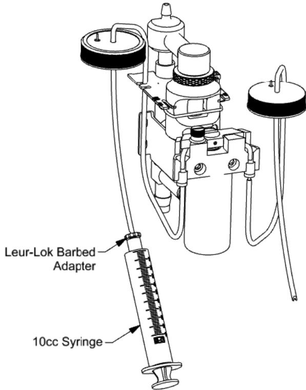
Figure 6: Check Valve Flushing
