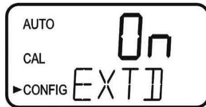
If extended settings are set to **OFF**, pressing the ↵ button will save all settings and the CLX-Ex2 will automatically return to the normal **AUTO** mode of the instrument.
