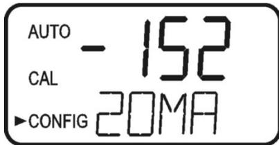
When complete with the 20mA adjustment, press the ← button to exit to AUTO mode and save all configuration settings.
