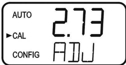
5. The screen will show the current reading on the CLX-Ex2. Using the  $\blacktriangle$  and  $\blacktriangledown$  buttons adjust the reading to agree with the laboratory method or portable photometer.
