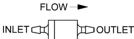
Figure 5: Inline check valve
