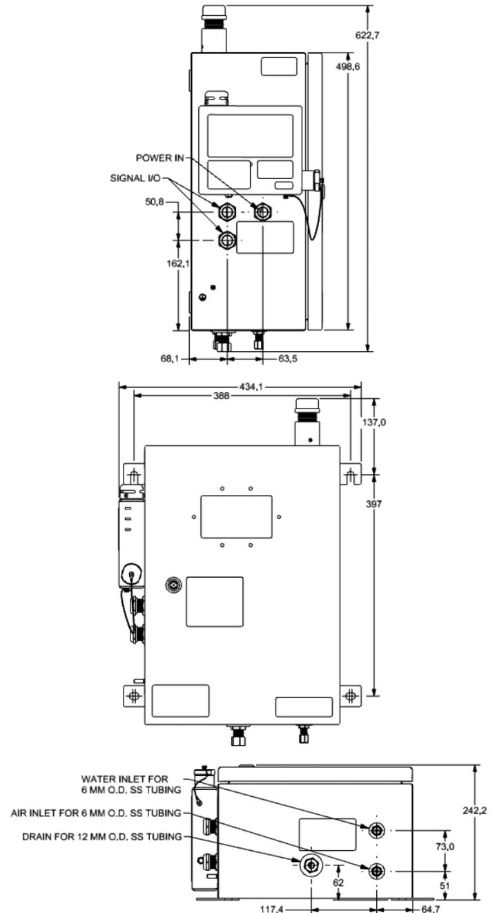
**Figure 4: Overall Mounting Dimensions of the Instrument**
