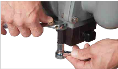
3. Use the two wrenches to tighten the hardware securing the sensor to the valve.
