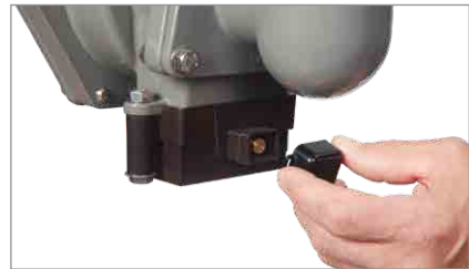
4. Remove the dust cover from the sensor.
