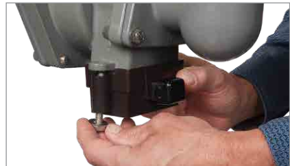
2. For each side of the sensor, put the washer on the head of the bolt, thread the bolt from the bottom, and hand-tighten the nut to the bolt.
