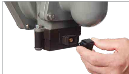
4. Remove the dust cover from the sensor.
