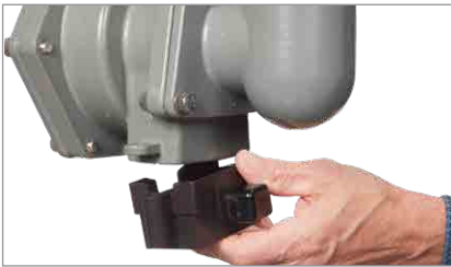
1. Position the flood sensor on the relief valve.
