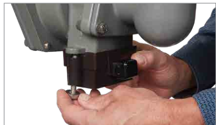
2. For each side of the flood sensor, put the washer on the head of the bolt, thread the bolt from the bottom, and hand-tighten the nut to the bolt.
