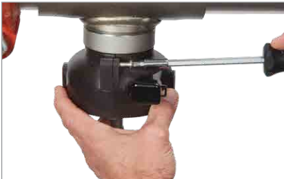
3. Insert the bolts and tighten.
