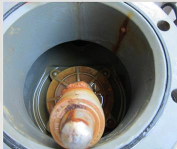
These images taken after 16 months in the same application as above shows little to no corrosion. Any corrosion resulting from a breach in coating has not spread.
