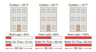
In order to calibrate the control to the heat loss rate of a particular building, the installer is required to enter the following heating curve settings:
