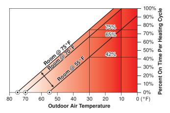
When an indoor sensor(s) is connected to the control, the Room setting becomes a Room Target temperature. The control measures the current air temperature in the room using the indoor sensors. The control then automatically shifts the heating curve so that the measured room temperature reaches the Room Target temperature.
