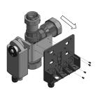
11. Loosen the 4 screws and remove the back of controller base from the metal valve bracket.
