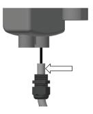
10e. Slide metal sheathing to remove from wire.
