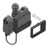
19. Position the front cover onto the unit, then snap it in place.
