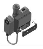
18. Put the wiring cover back on and tighten the 2 screws.
