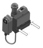
4. Using a screwdriver, loosen the 2 screws at the front of the wiring cover.
