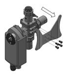
12a. Loosen 4 screws in center of metal valve bracket and remove bracket from valve body.
