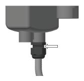
14b. At the actuator end of the cable, thread the black nipple to the actuator.
