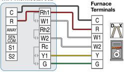
The WiFi Thermostat 562 operates a first stage radiant floor and a second stage furnace for heating, and an air conditioner for cooling.
