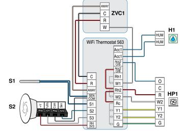
The WiFi Thermostat 563 operates a two-stage water-to-air heat pump for heating and cooling. The heat pump absorbs or rejects heat to a hydronic water loop that is heated by a boiler and cooled using a cooling tower to maintain a constant temperature of approximately 70°F (21°C).
