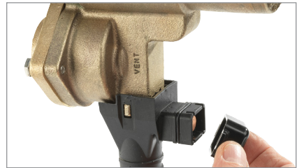
4. Remove the dust cover from the sensor.
