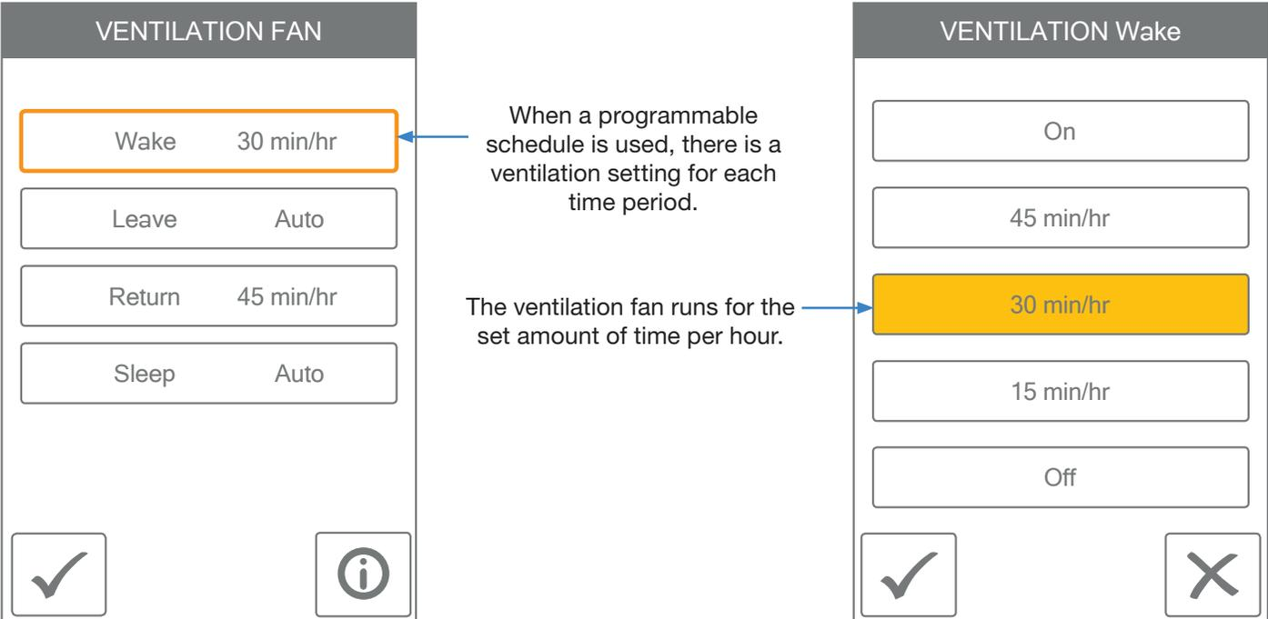
The "VENTILATION FAN" screen has a dark header and four white buttons: "Wake 30 min/hr", "Leave Auto", "Return 45 min/hr", and "Sleep Auto". At the bottom are a checkmark button and an information button.
