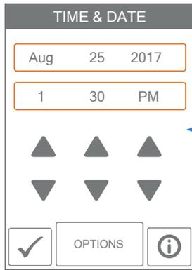
The time and date can be manually set by highlighting a field and then using the ▲ or ▼ buttons.
