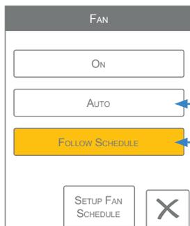
The fan is normally off when set to auto but turns on when needed for the heating or cooling equipment.
