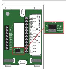
The thermostat includes three relay power jumper connectors located below the wiring hole.
