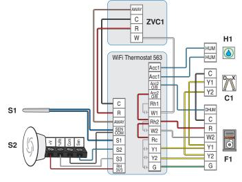
The WiFi Thermostat 563 operates a first stage radiant floor and a two-stage air-to-air heat pump for heating, cooling, and dehumidification, a backup electric heater, and a humidifier.
