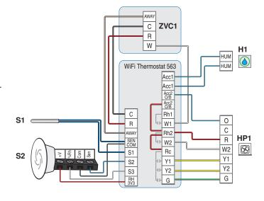
The WiFi Thermostat 563 operates a two-stage water-to-air heat pump for heating and cooling. The heat pump absorbs or rejects heat to a hydronic water loop that is heated by a boiler and cooled using a cooling tower to maintain a constant temperature of approximately 70°F (21°C).
