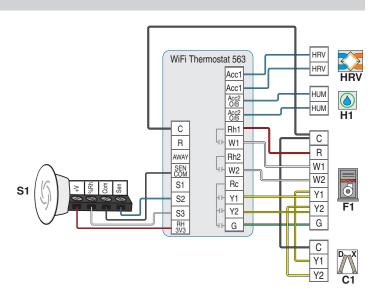
The WiFi Thermostat 563 operates a first stage radiant floor and a second stage fan coil for heating, and two-stage air conditioner for cooling and dehumidification, and a humidifier.
