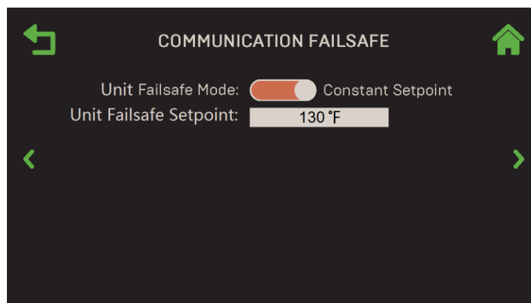
Figure 4-57: Comm & Network : Communication Failsafe Screen
