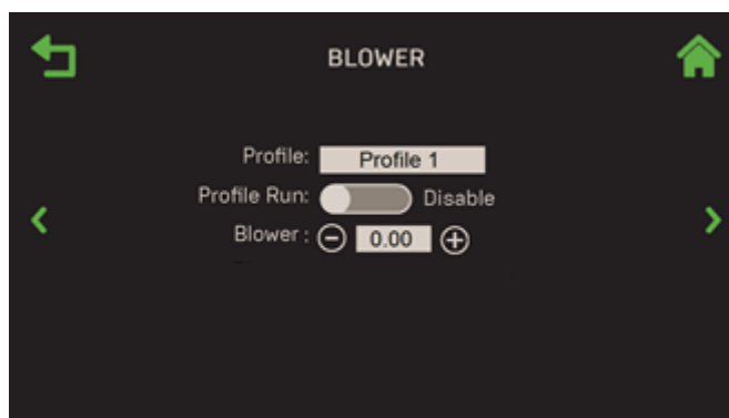
Figure 3-13: Subsystems: Blower Screen
