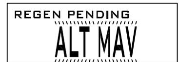
*STAND BY* is displayed in alternator systems when a valve is in standby mode. The name of an active MAV will also be indicated in this display.
