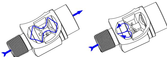
Full flow during standard operation, providing the supply needs for the gas appliance
