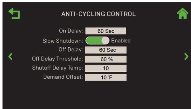
Figure 6-83 : Fire Control : Standalone Anti-Cycling Controls
