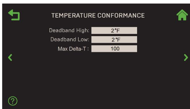
**Figure 6-77 : Temperature Control : Temperature Conformance**
