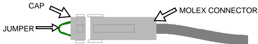
**Figure 2-21: Sequencing Isolation Valve Molex Connector and Jumper Wire**
