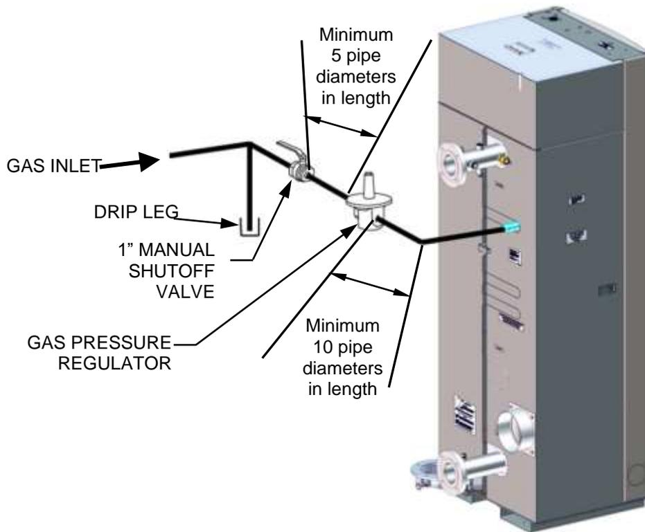
**Figure 2-8a: BMK750-1000 Gas Regulator and Manual Shut-Off Valve**
