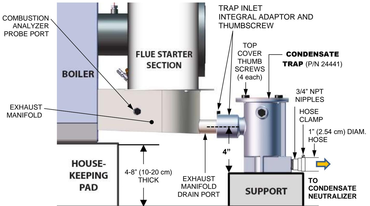
Figure 2-7b: BMK1500 – 6000 Sample Condensate Trap Installation
