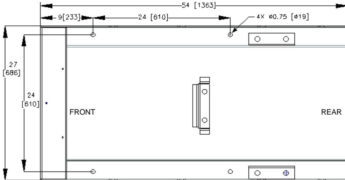
**Figure 2-2c: BMK2500-3000 Anchor Bolt Locations**
