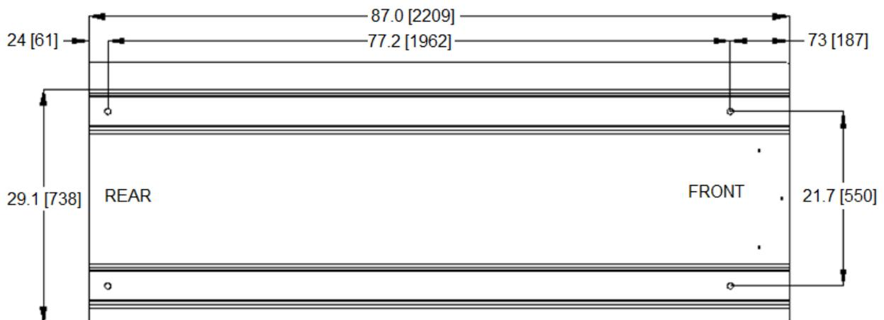
**Figure 2-2e. Benchmark 5000-6000 Anchor Bolt Locations**
