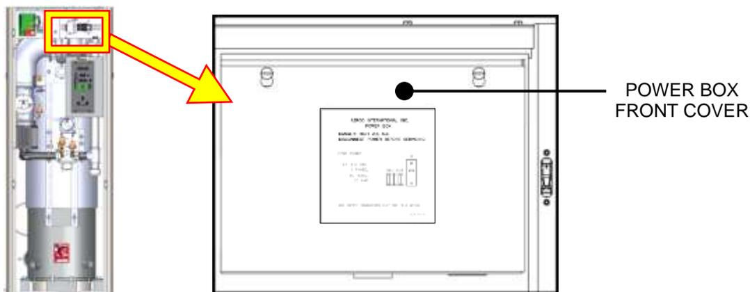
**Figure 2-9b: BMK1500 – 6000 Power Box with Closed Cover**
