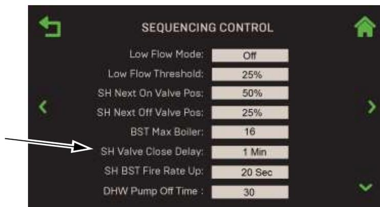
**Figure 2-19: Sequencing Control Screen**
