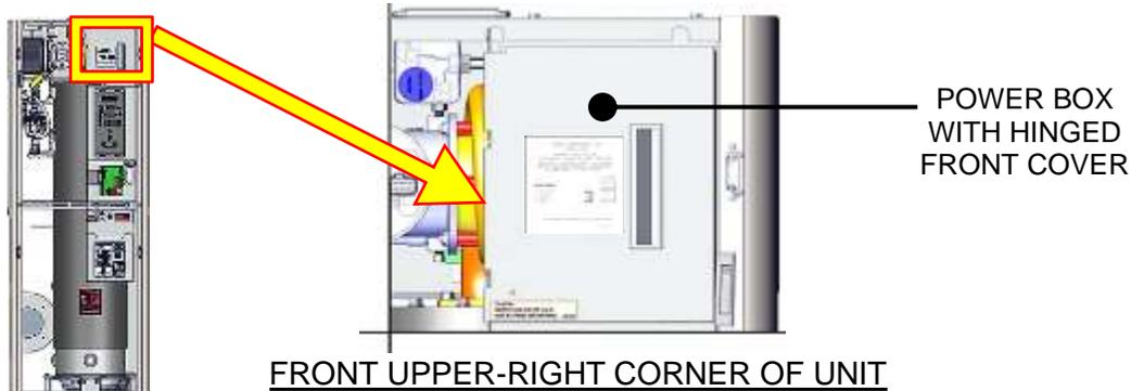
**Figure 2-9a: BMK750-1000 Power Box with Closed Cover**
