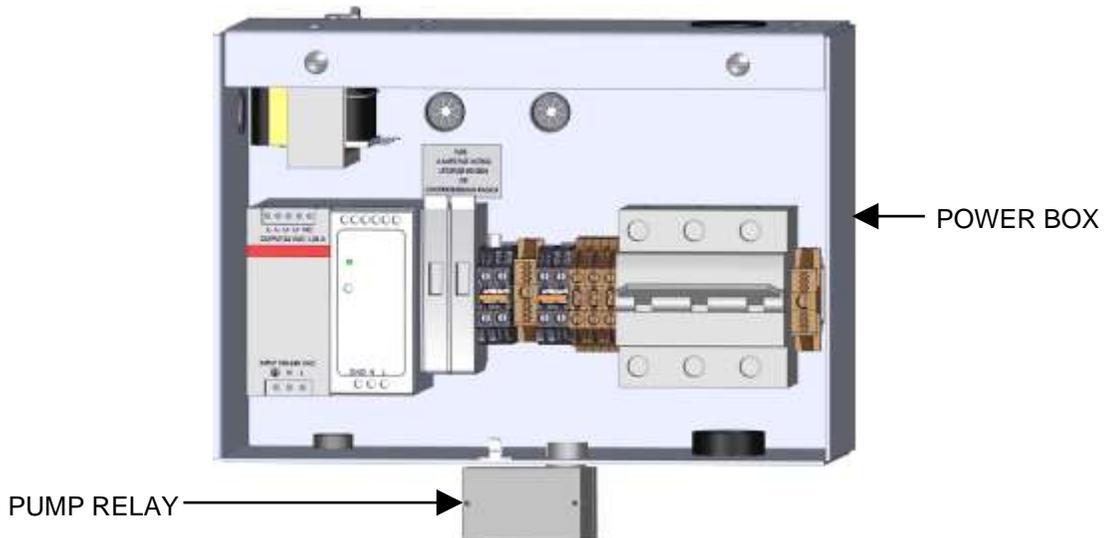
**Figure 2-16b: BMK1500 – 6000 Pump Relay Location (BMK2500/3000 Shown)**
