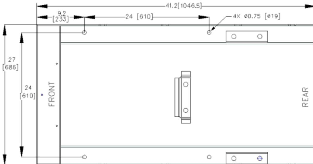
**Figure 2-2b: BMK1500-2000 Anchor Bolt Locations**
