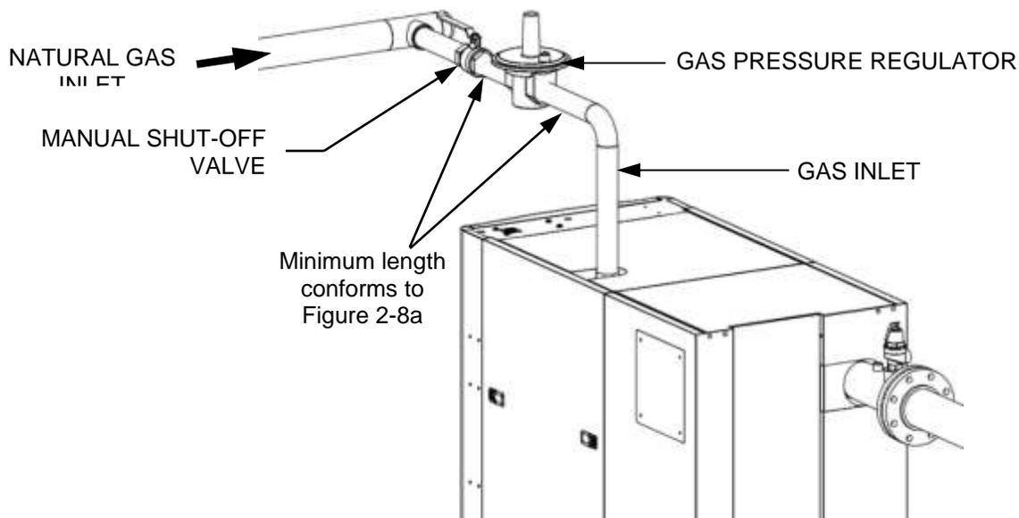
**Figure 2-8c: BMK1500 – 5000N Gas Regulator and Manual Shut-Off Valve**
