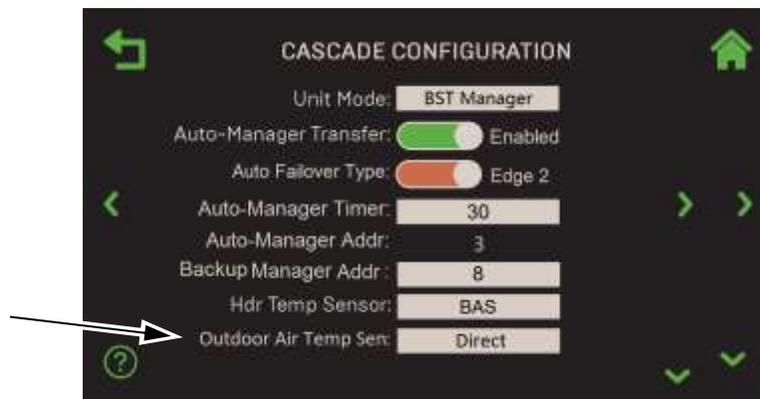
**Figure 2-13: Cascade Configuration Screen**
