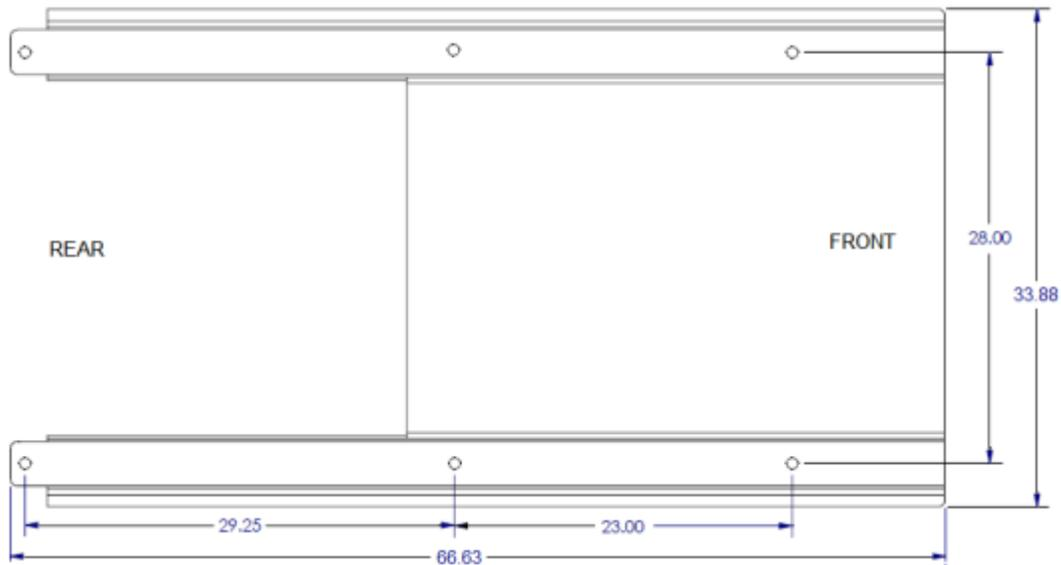
**Figure 2-2d: BMK4000-5000N Anchor Bolt Locations**
