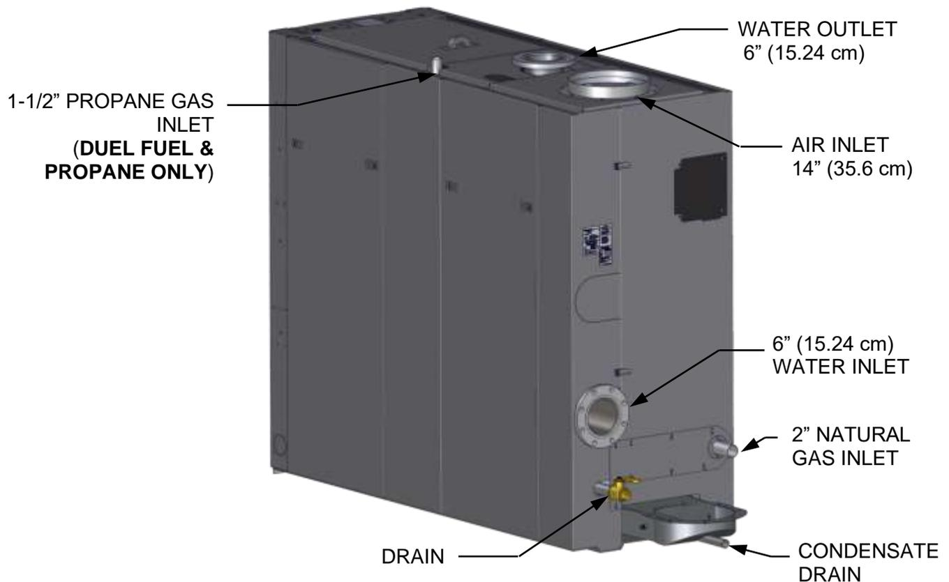
*Figure 2-5c: BMK5000-6000 Supply and Return Locations (DF Model Shown)*
