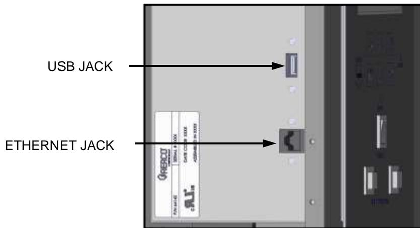
*Figure 3-2: Edge Controller – Left Side View*
