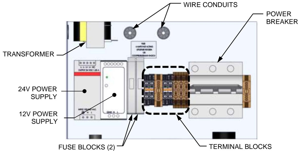
**Figure 2-10c: BMK2500 – 6000 Power Box Internal Components**
