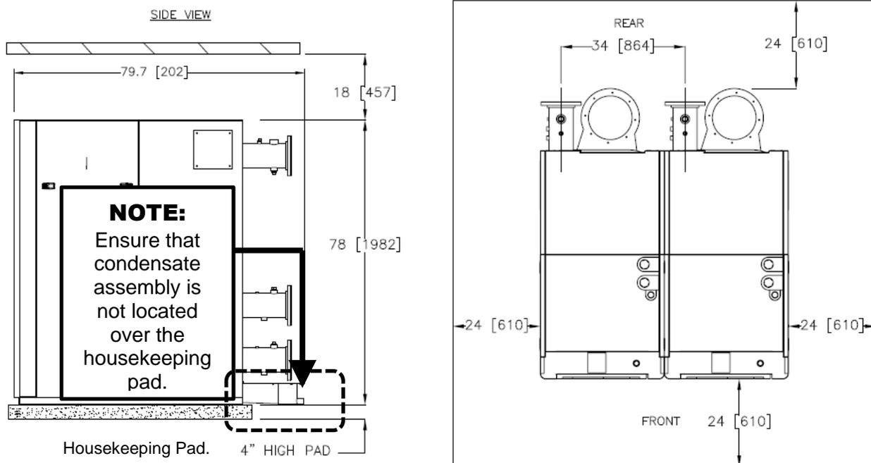
Figure 2-1d: BMK4000-5000N Clearances
