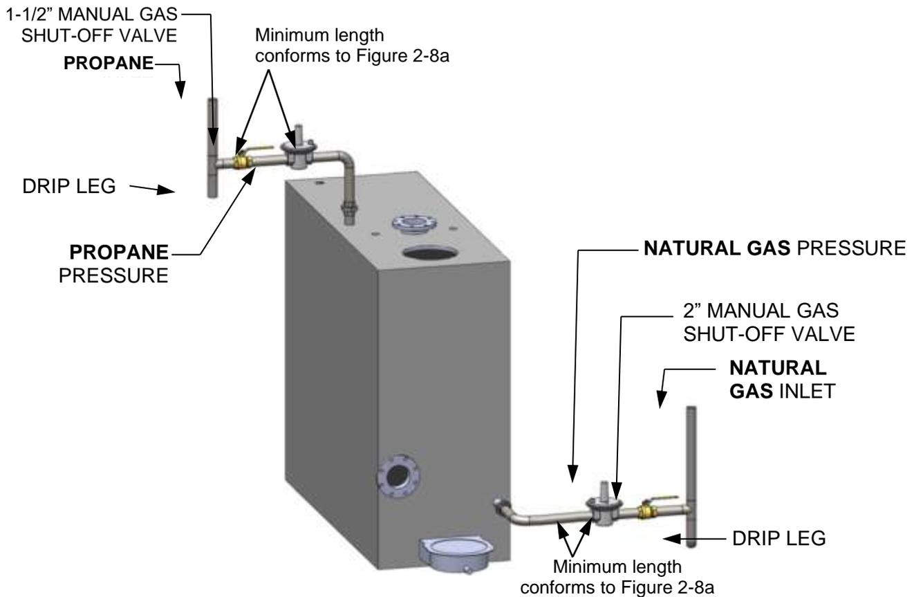
**Figure 2-8e: BMK5000-6000 Manual Gas Shut-Off Valve Location – Dual Fuel**
