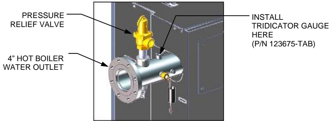
**Figure 2-6b: BMK1500 – 5000N P&T Relief Valve Location**
