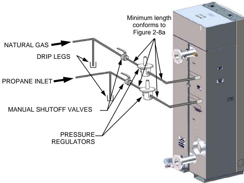
**Figure 2-7b: BMK750-1000 Dual Fuel Gas Regulator and Manual Shut-Off Valve**
