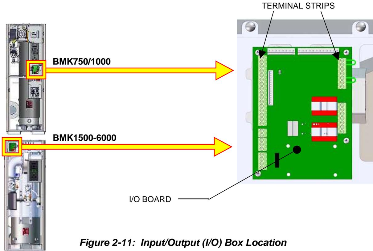
**Figure 2-11: Input/Output (I/O) Box Location**
