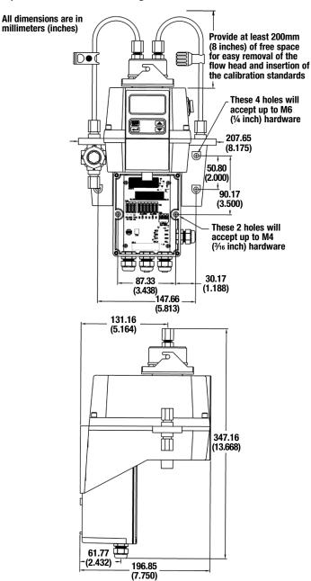
Figure 3: Overall Mounting Dimensions of the Instrument
