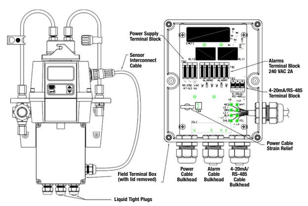
Figure 5: Electrical Connections for the Instrument
