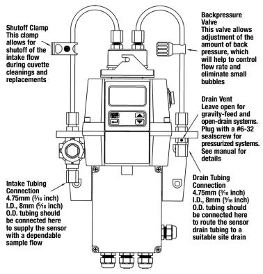
Figure 4: Recommended Plumbing for the Instrument
