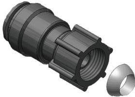
AquaLock connectors utilize a swivel nut with NPS straight threads and a cone seal. This allows the installer to thread onto NPT, NPS, BSP and most 1/2" male threads without tools or thread sealant. Simply thread on, hand tight, for a zero-leak seal.
