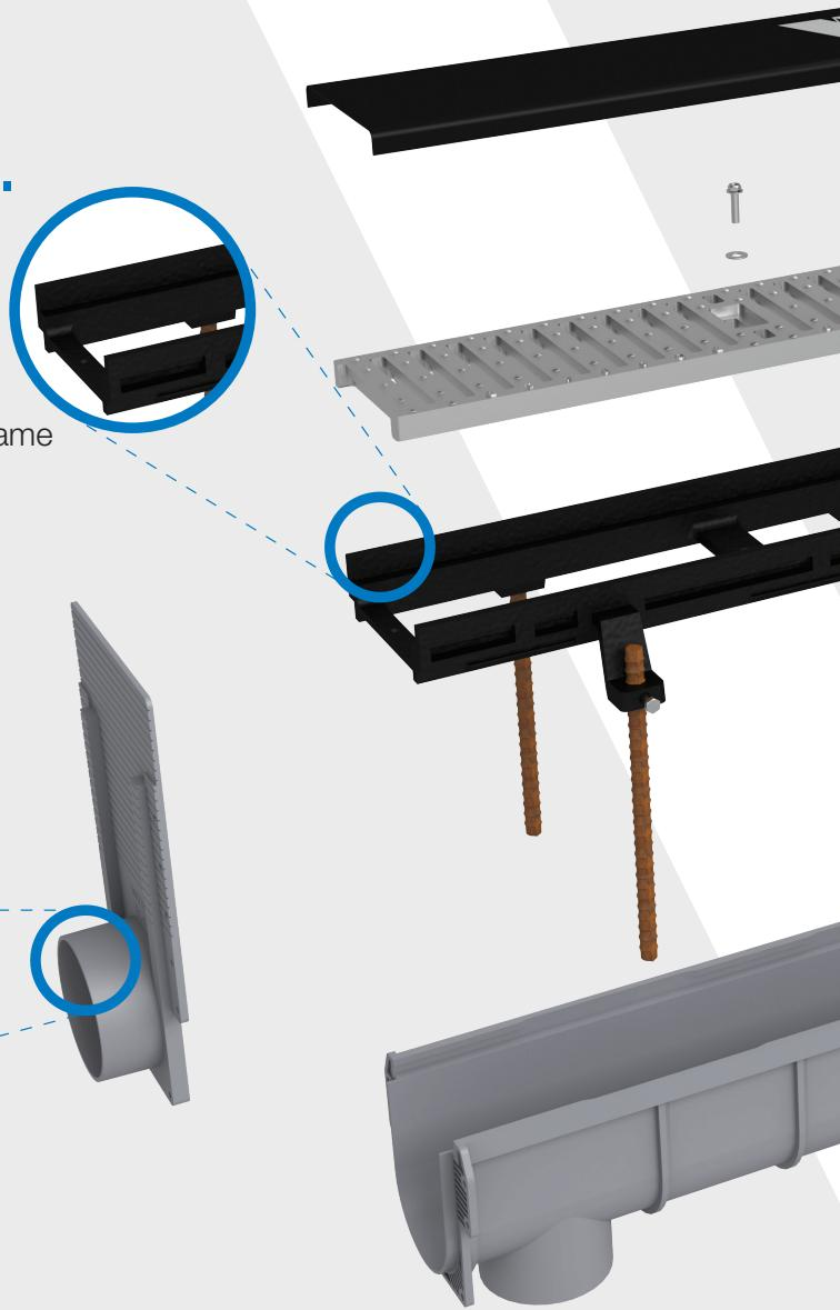
**Structural Stability** — Patented frame-anchored design ensures that drains go in straight and stay straight. Channels lock longitudinally outside the structural frame and cannot pinch, twist, or float with the concrete pour.
