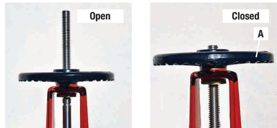
1. Slowly rotate shutoff valve #2 handle to the closed position. Stem concealed (A).
