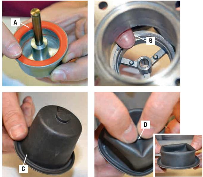
1. Place the piston assembly (A) into the diaphragm (B), making sure the diaphragm lays flush on the bottom of the piston assembly with no wrinkles or tears in the diaphragm.
