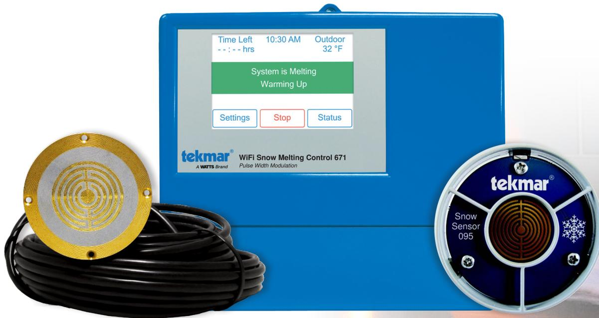
The WiFi Snow Melting Control 671 operates hydronic and electric heating equipment designed to melt snow and ice from roads and walkway surfaces. The control works with the tekmar Snow/Ice Sensor 090 or Snow Sensor 095 to automatically detect snow or ice and operates a single boiler, steam valve, or electric cable to supply heat to the slab.
