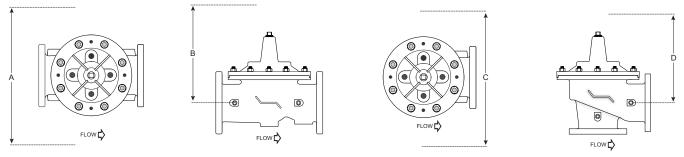
The following tables detail the recommended minimum valve servicing dimensions.
