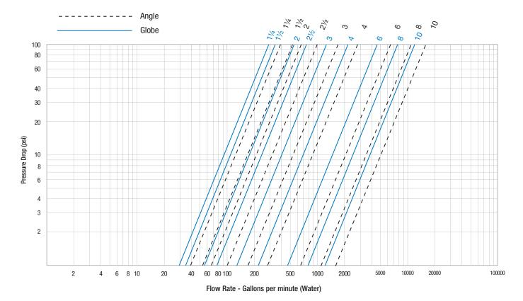
The  $C_V$  factor of a value is the flow rate in US gpm at  $60^{\circ}$  F that will cause a 1 psi drop in pressure. The factors stated are based upon a fully open valve.
