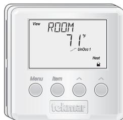
The tekmar Room Temperature Unit (RTU) 062 consists of an air temperature sensor, a liquid crystal display (LCD) and four buttons. These buttons and the LCD are used to set and view the desired room temperature. The RTU's LCD displays the current room temperature, the outdoor air temperature and a number of other items.
