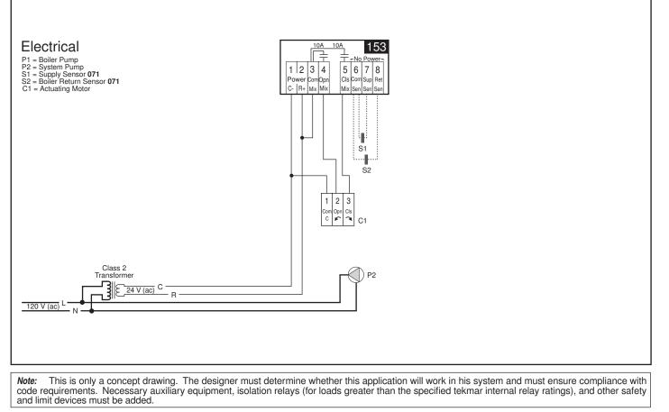
Power 24 V (ac) ± 10% 50/60 H 24 V (dc) ± 10% 0.03 A Relay 240 V (ac) 10 A 1/3 hp
