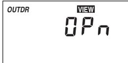
The control is no longer able to read the outdoor sensor due to an open circuit. In this case the control assumes an outdoor temperature of 32°F (0°C) and continues operation. Locate and repair the problem as described in the Testing section. To clear the error message from the control after the sensor has been repaired, press the **Item** button.
