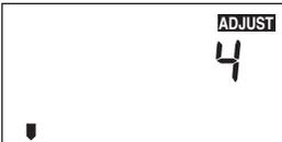
Press and release the **Item** button to advance to the *Terminal Unit* adjustment. Use the ▲ or ▼ button to select the desired terminal unit. The terminal unit number corresponds to the type of terminal that is being used to heat the space. The table below lists the terminal units and their default values.
