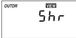
The control is no longer able to read the outdoor sensor due to a short circuit. In this case, the control assumes an outdoor temperature of 32°F (0°C) and continues operation. Locate and repair the problem as described in the Testing section. To clear the error message from the control after the sensor has been repaired, press the **Item** button.
