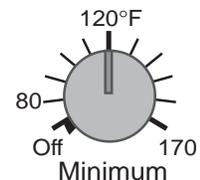
Overheating of buildings in warm weather will occur where minimum boiler temperatures are required, unless the building has either a mixing system to reduce system supply water temperatures to below boiler minimums, or some sort of room temperature control and zoning system. Zone controls from tekmar, when used in these applications, will provide room temperature feedback information to this control, allowing it to shift the heating curve for maximum comfort and energy savings.
