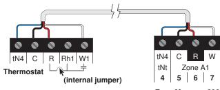
End Switch (from Mixing Module, Zone Valve, etc.)
