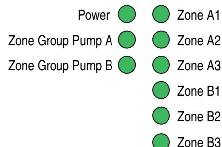
Nine LEDs to provide the status of the 337's outputs.
