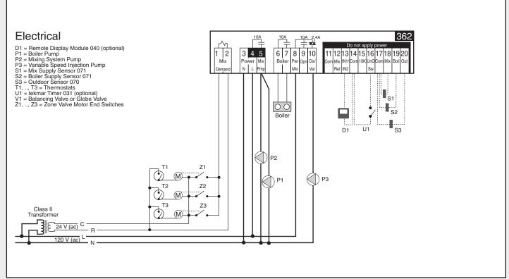
The Mixing Control 362 provides full outdoor reset to three (or more) mixed zones. The output of the variable speed injection pump is modulated to mix the water temperature to the zones and protect the boiler from flue gas condensation. The boiler operates at the required temperature in order to satisfy the load. An optional Remote Display Module (RDM) provides remote adjustment and monitoring.
