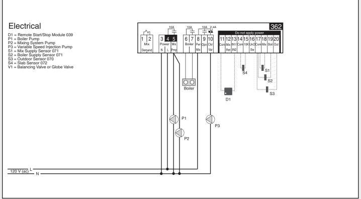
The Mixing Control 362 provides a single zone snow melting system. The heat source is sized and dedicated to the snow melting system. The output of the variable speed injection pump is modulated to protect the boiler from flue gas condensation.
