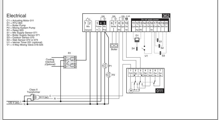
The Mixing Control 362 provides full outdoor reset to a single mixed zone. The single mixed zone temperature is controlled through a Room Temperature Unit (RTU) 063 and can be configured for slab or indoor air and slab temperature control. The position of the mixing valve is modulated to provide a mixed supply water temperature to the mixed zone and to protect the boiler from flue gas condensation.
