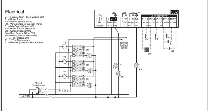
The Mixing Control 362 provides a single zone snow melting system. The output of the variable speed injection pump is modulated to mix down the boiler supply fluid temperature to protect the slab from thermal stress and to protect the boiler from flue gas condensation.
