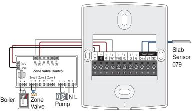
The 521 operates a single hydronic heating zone by operating a zone pump. The boiler is operated by an end switch. An optional Slab Sensor 079 can be installed for radiant floor heating applications. The temperature is automatically adjusted by an optional programmable schedule. Optimum start learns the heat up rate of the room and starts the heating early so that the room is warm at the time set on the programmable schedule.
