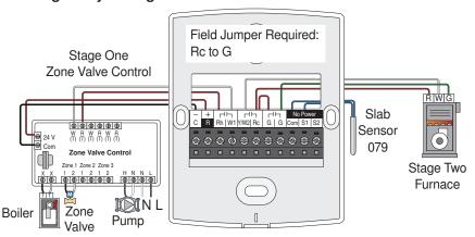
The 521 operates a hydronic fan coil for heating and operates an air conditioner for cooling. The temperature is automatically adjusted by an optional programmable schedule. The fan is operated together with the fan coil or air conditioner or can be manually set on to provide air circulation in the building.
