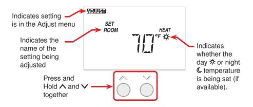
This thermostat has access levels. It will typically be installed and programmed by a heating professional and then locked in a "User" access level. System critical settings will not be available for adjustment. For more information on these settings, please consult your installing contractor or this product's Installation and Operation Manual. The following pages describe the settings available to the "User".
