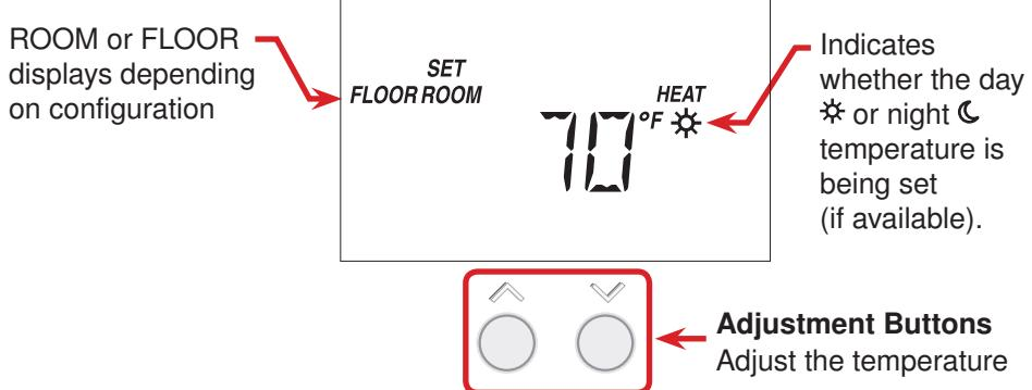
You will be adjusting the temperature of the current operating mode. To adjust temperature settings that are not shown on the screen, you must enter into the Adjust Menu as described in the "Adjust Menu" section. There may be other symbols on the screen that affect thermostat operation. Please see the "Display Symbols" section for a description of each symbol.
