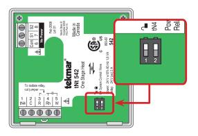
*Note:* The tN4 System Control's Lock/Unlock DIP switch overrides the Lock/Unlock DIP switch on the 542. Set the tN4 System Control's Lock/Unlock DIP switch to the Unlock position before Access Levels can be changed on the thermostat.
