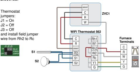
The WiFi Thermostat 562 operates a first stage radiant floor and a second stage fan coil for heating, and an air conditioner for cooling.
