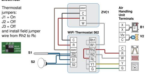
The WiFi Thermostat 562 operates a first stage baseboard/radiator and a second stage fan coil for heating, and an air conditioner for cooling.
