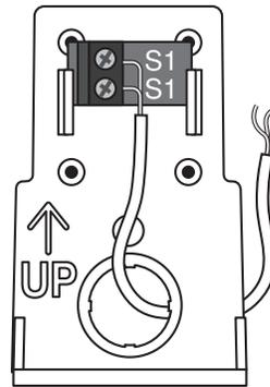
Wires from outdoor sensor and sensor common terminals on tekmar control
