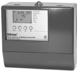
The Snow Detector & Melting Control 667 is designed to control a single zone snow melting system. The control automatically adjusts the mixed supply water to the snow melting system by controlling a single boiler and a variable speed injection pump. The snow melting system may be started manually or automatically through the use of a Snow/Ice Sensor 090. Standard features include pump exercising, slab and boiler protection, and many other useful items.
