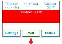
Press Melt button to start melting operation
