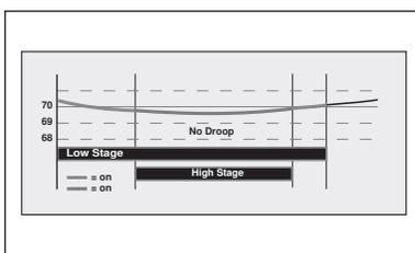
To provide proper two staging heating and an accurate room temperature, PID (Proportional, Integral, Derivative) control logic should be used. With PID control logic, the operation of the second stage depends on how far
