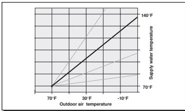
The full range of temperatures required through a heating season can be provided with a non-condensing boiler together with a mixing device. The mixing device provides different water temperatures based on the outdoor
