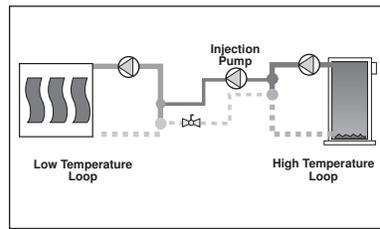
Variable Speed Output is used to vary the speed of a permanent capacitor, impedance protected pump motor of less than 1/6 hp. The pump is piped to inject hot water at different rates from a high temperature loop into a
