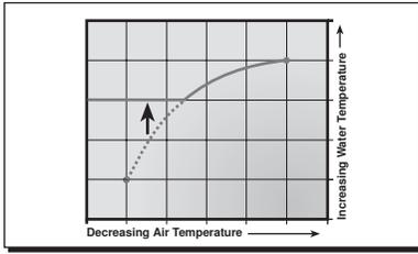
Most setpoint loads in a heating system operate year round and often at temperatures above the reset operating temperature. When the setpoint load requires heat, this overrides the Warm Weather Shut Down and
