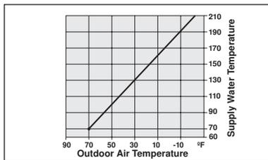
In order to properly control a hot water heating system, the heat supplied to a building must equal the heat loss from the building. The heat loss is dependent on the outdoor temperature. It is therefore necessary to reset
