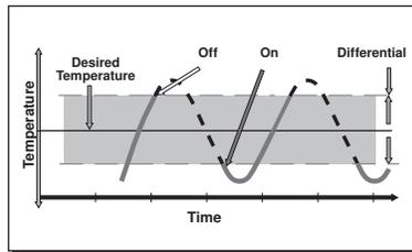
An on / off device, such as a boiler, must be operated with a differential in order to prevent short cycling. When the supply water temperature drops below the bottom rail of the differential, the device is turned on. The device is
