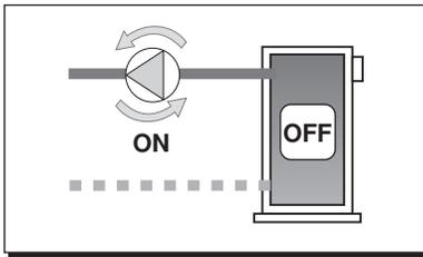
When a boiler is turned off some heat remains in the mass of the boiler. If the flow through the boiler is stopped at the same time the boiler is shut off, the residual heat is lost. Therefore, after operation of the boiler the residual
