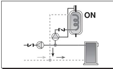
When DHW priority is used, the water temperature within the heating terminals may have cooled down significantly lower than the boiler operating temperature. When the DHW operation is complete the DHW pump will
