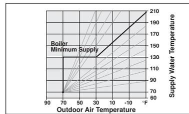
Most boilers require a minimum supply water temperature in order to prevent corrosion from flue gas condensation. The control should therefore only modulate the boiler supply water temperature down to the
