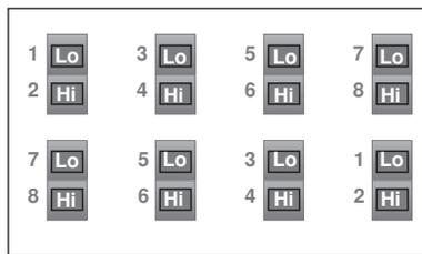
Many boilers or water heaters have two stage burners. The control must therefore stage the operation of the burner by first firing the lo fire and then the hi fire. If equal run time rotation is desired, the control must now rotate
