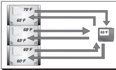
In systems where tenants have control of the space temperature, a central zone control with a temperature Adjustment Range Limit can allow the building owner to limit the maximum space temperature in the zones. This
