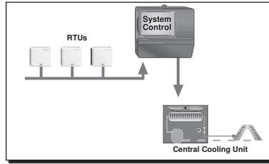
Heating / Cooling Interlock prevents the system from heating and cooling simultaneously. When the heating Room Temperature Units (RTU) have been satisfied for a period of time, the control allows for the cooling unit to
