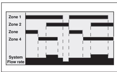
In a multiple zone system there can be sudden load changes due to multiple zones opening and closing. Zone load coordination staggers the operating times of each zone in order to maintain a relatively constant flow
