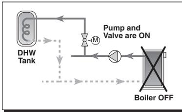
During DHW operation, the boiler temperature is normally raised above 180°F (82°C). Once the DHW tank is satisfied, the residual heat from the boiler may be wasted if there is no other call for heating. This residual
