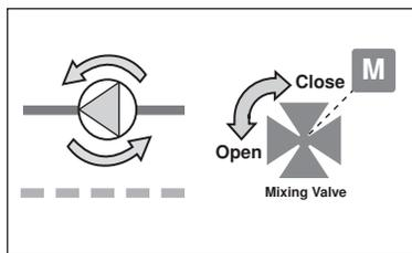
The control operates the system components every three days for a few seconds to help prevent corrosion build up and the subsequent seizure. The control must ensure that during exercising no heat is supplied to the zones
