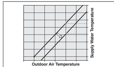
When setback is required, the water temperature to the system should be decreased to provide less heat into the space. tekmar Reset Controls shift the heating curve down in order to provide lower water temperatures
