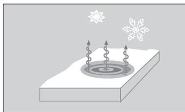
Snow / ice detection is used to automatically start and stop a snow melting system. When there is snow on the sensor, the sensor melts the snow / ice, detects the moisture and allows the control to start the melting process.
