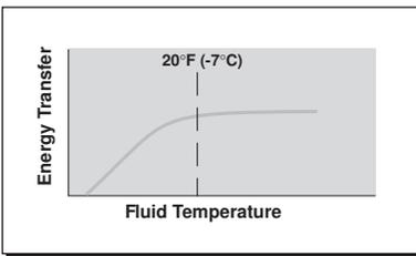
A glycol solution in snow melting systems increases viscosity at colder temperatures. This reduces the system flow rate and heat transfer. In order to compensate for these changes, the control automatically raises
