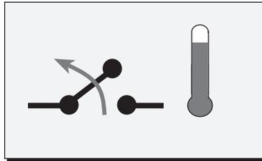
When the slab and outdoor temperatures are warm enough, the snow melting system should automatically turn off. The Warm Weather Cut Off (WWCO) function automatically shuts off the system when snow melt-
