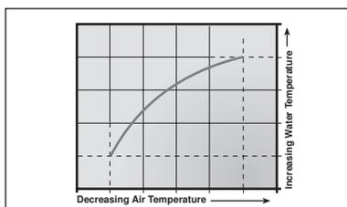
A Characterized Heating Curve is a more accurate method of outdoor reset. Each type of terminal unit delivers heat into a building with different proportions of radiation, natural convection and forced convection. With a Characterized Heating Curve, the control takes into account both the outdoor temperature and the type of terminal unit in order to determine the best water temperature for the system.
