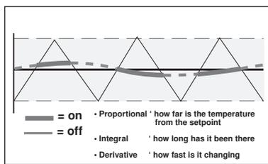
To prevent excessive room temperature swings and offset, PID (Proportional, Integral, Derivative) control logic should be used to control the zone temperature. With PID control logic, the control operates the zones
