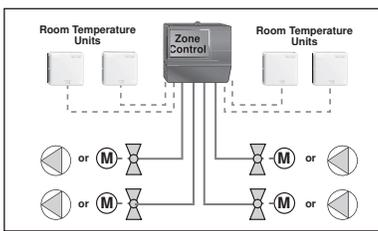
Integrated Zoning allows one central zone control to control multiple zones in a heating system using state of the art micro-processor technology. Sensors throughout the building are connected to the zone control and provide
