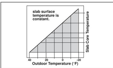
In snow melting systems the slab sensor is normally an inch below the slab surface. When the outdoor temperature suddenly drops, the sensor does not register this change immediately and surface freeze up could
