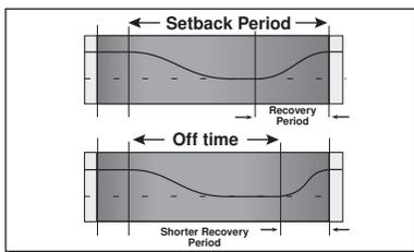
By increasing the supply water temperature during the recovery period before the end of the setback schedule, faster pick up times can be achieved. This allows for longer setback periods and therefore more energy savings
