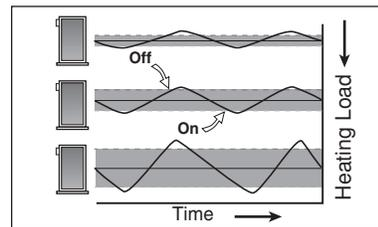
In order to decrease temperature swings and increase boiler efficiency, this function automatically changes the on / off differential of the boiler based on the heating load. As the load increase, the differential will decrease to
