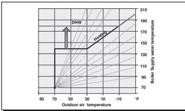
Most indirect fired DHW tanks require a boiler supply water temperature of at least 180°F (82°C) in order to transfer sufficient heat. If the boiler is also using a reset control for space heating, the water temperature may
