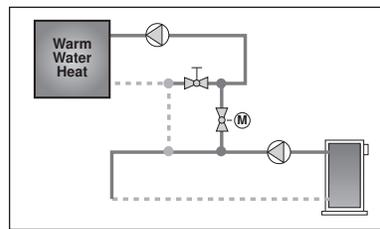
On / Off Injection output is used to operate an on / off device, such as a valve or a pump, in order to inject heat into a constant circulating low temperature loop. This type of mixing requires a differential in order to prevent
