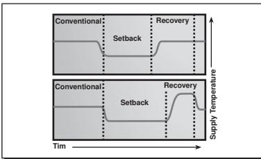
When combining setback with outdoor reset, the morning recovery period can be extremely long. By increasing the supply water temperature after the end of the setback period, a faster pick-up can be achieved. This
