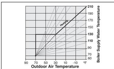
A boiler is controlled by turning it on and off. In applications where Outdoor Reset is used, the boiler temperature can be lowered based on the outdoor temperature. Resetting the boiler temperature is limited by the
