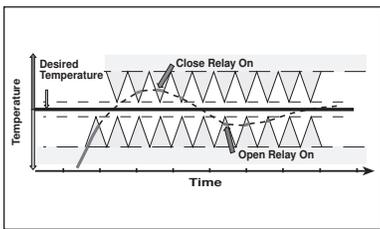
Floating action is an output used to modulate the position of an actuating motor and mixing valve. Floating Action either provides power to drive the motor further open or closed. If no power is supplied, the
