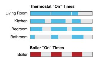
With synchronization, the cycle start times are coordinated between zones to allow for longer on & off times. Reducing equipment short cycling prolongs the boiler life & improves system efficiency.
