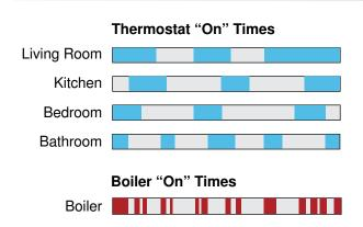
Without synchronization, the boiler is at the mercy of each zone. Non-communicating thermostats short cycle the boiler to achieve independent targets rather than systemwide goals. Boiler operation is inefficient & unreliable.
