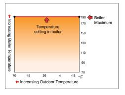
Without Outdoor Temperature Reset, the boiler water temperature is the same for the entire heating season.
