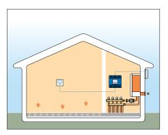
When the thermostat calls for heat, the tekmar control operates the boiler to provide a 'reset' water temperature.
