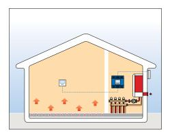
On colder days the boiler water temperature is higher.
