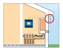
tekmar controls with Outdoor Temperature Reset monitor the outdoor temperature.
