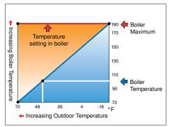
With Outdoor Temperature Reset, the boiler temperature is continually adjusted to match the heat loss of the building.
