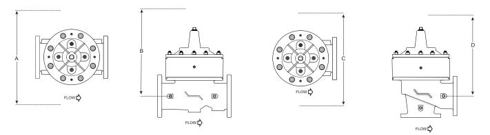
The following tables detail the recommended minimum valve servicing dimensions.
