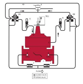
able floor drain. The valve closes at an adjustable rate, gradually reducing pumping pressure. Rate of valve closure is controlled by the adjustable closing speed control, which restricts the speed at which fluid and pressure evacuate the power chamber. When the valve reaches the closed position, the limit switch is actuated, turning the pump off.
