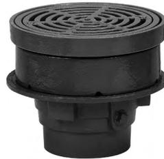
Watts FD-320-SET epoxy coated cast iron area drain with anchor flange, membrane clamp with weepholes, 8"(203) diameter adjustable top, loose set heel proof ductile iron grate supported by bucket, and no hub connection (standard).
